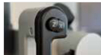
Pneumatic selective clamping in X and Z
