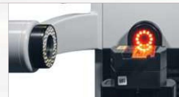
Center height measuring camera on optics carrier with LED ring light
