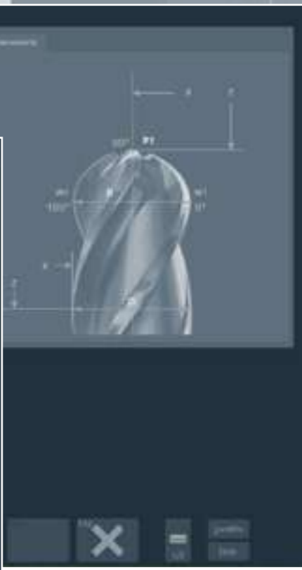
Analyzing the radius contour of full radius milling cutters in adjustable angular increments. (measuring program 137)
