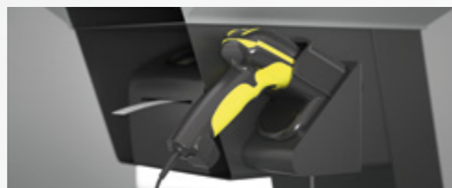
Tool identification via scanner on the »cockpit« control unit
